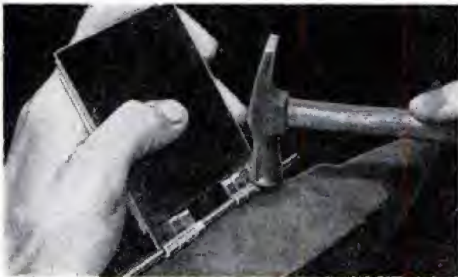
Brazing rod, which serves as hinge pin, is used in forming eyes in ends of tabs by tapping metal around it
